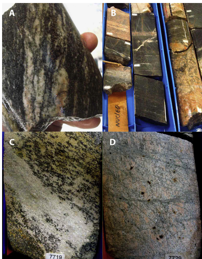
Fig. 5. Photographs from some of the drilling-core samples analyzed during the present study. (a) Migmatitic gneisses from the Payara-1 well, (b) Stromatic migmatites injected by granitic sills from the Mandur-2 well, (c) Metasedimentary Qz-Fsp migmatites from the Caiman-3 well, and (d) Leucocratic gneisses that crosscut the metamorphic foliation of the migmatites in the Caiman-3 well.
